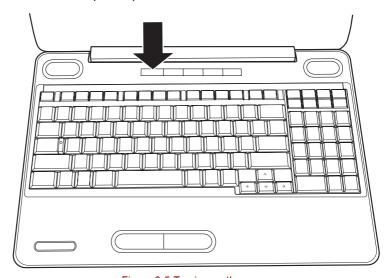
Figure 3-5 Turning on the power
